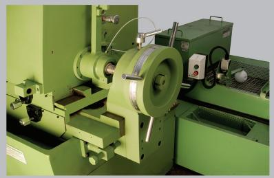
Scarlo infeed design has a swivel slide for work's taper adjustments. Antifriction bearings between the swivel and middle slide are a standard feature on all machines. All machines are fitted with high precision ground ball screws in-line with the hand wheel for infeed movement.
