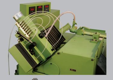
Apart from the above mentioned features, the CNC/PLC variant for Grinding Wheel Dresser is equipped with precision ball screws for both axis, traverse motion and diamond ram movement. The dresser variants can be one or two axis servo as required by the end user.
