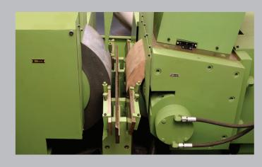
Scarlo Regulating Wheel Dresser has dovetail slide design with hydraulic cylinder for traverse motion. The dresser ram is spring loaded and supported on a cam. The unit is a Swivel type regulating wheel truing unit which is independent from regulating wheel swivel. Diamond advance least count is 0.02mm.
