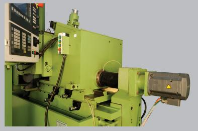
Scarlo CNC/PLC infeed design comes with swivel slide for work piece taper adjustments. Antifriction bearings between swivel and middle slide are a standard feature on all machines. All machines are equipped with high precision ground ball screw fitted in-line with bellow coupling and servo motor for infeed axis movement.
